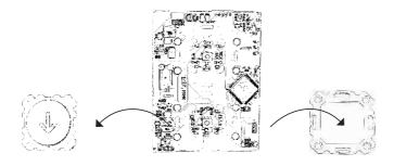
4 Turn the button around, so that it directs up. Place it back in the circuit borad with an angle, and turn it to its correct position.
