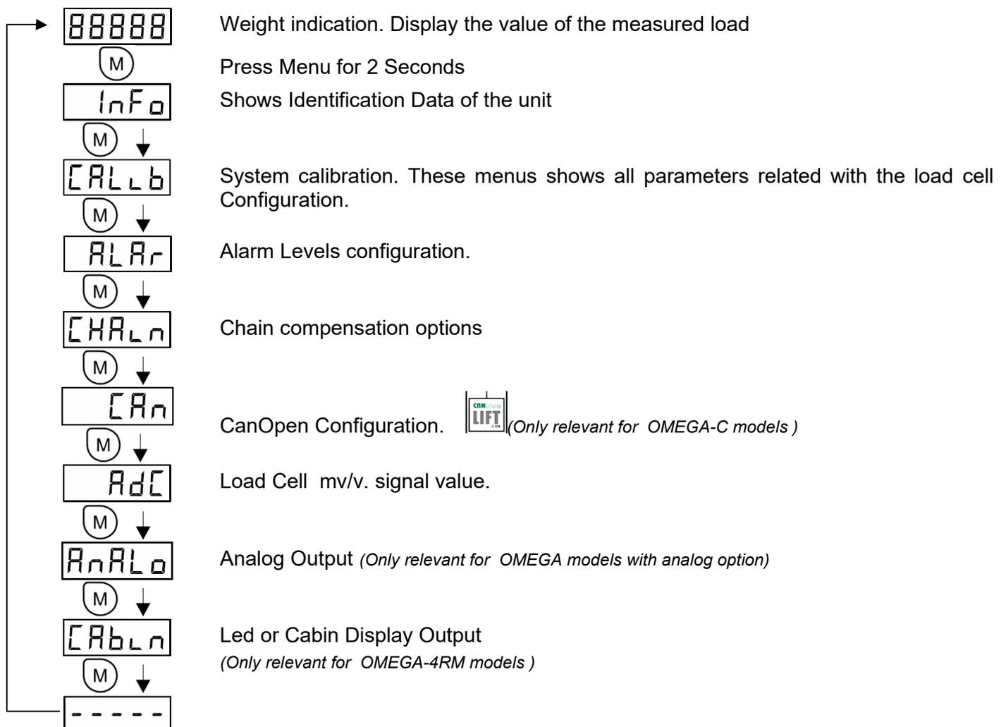
Pressing Menu for 2 seconds inside the internal navigation menu will end the menu navigation and return to Display the value of the measured load
