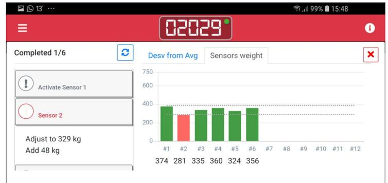
Following the suggested steps, you can apply the precise load to each rope to perform the whole "wire rope tension" process, just in a few minutes.
