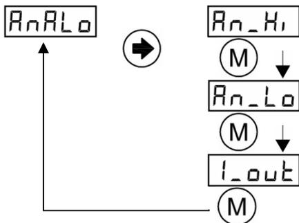
→ **Analog High:** Set the Load value desired (kg or Lb) To deliver the maximum analog output ( 10v or 20 ma)
