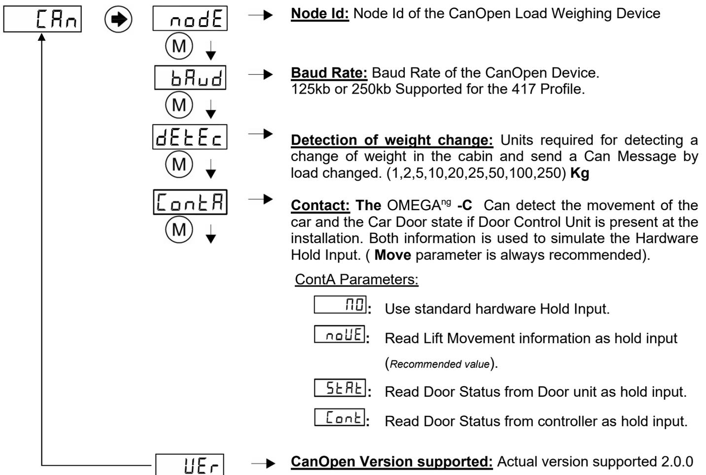
Bus Connection must be according application profile CiA-417 CAN high speed standard (ISO99-2) .
