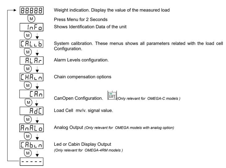
Pressing Menu for 2 seconds inside the internal navigation menu will end the menu navigation and return to Display the value of the measured load
